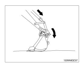
(10) To engage the quick coupler, release the quick coupler button on the right RCV lever.
